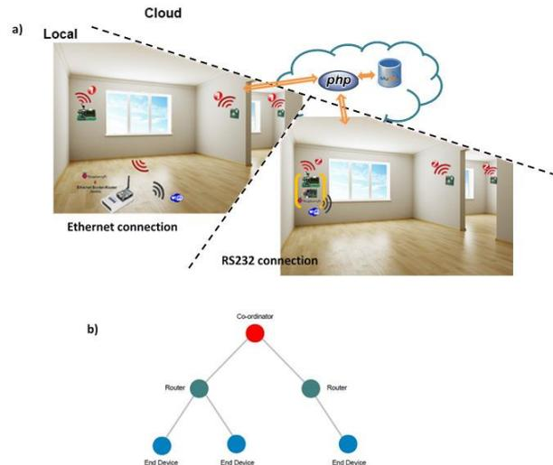
Fig 2. Distributed system for air quality a) indoor distribution of WSN nodes IEEE802.15.4 compatible, b) WSN topology – tree.
