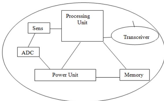
Fig. 1. Basic components of a smart sensor node in a Wireless Sensor Network.
